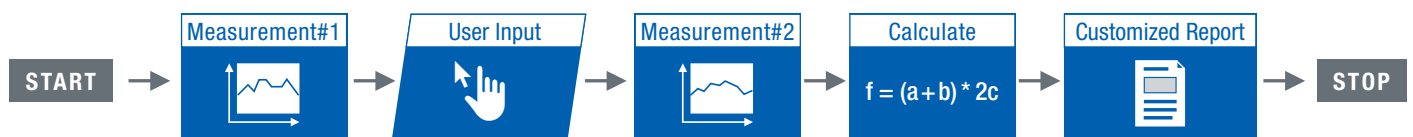
Example of an automated test sequence including operator input
