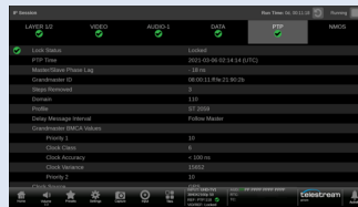
This display provides PTP syntax information including Grandmaster ID, Domain, Clock Class/ Accuracy/Variance. Priority 1 & 2 values along with message rates.
