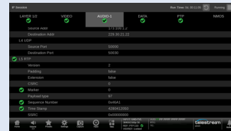
The Audio tab shows shows IP address, port number and RTP Layer 5 information such as Marker, Payload Type, Sequence Number and Timestamp.
